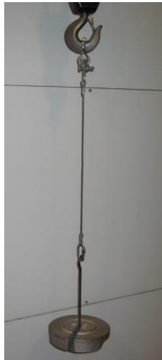
Figure 8: Free-hanging weight simulating material tension.
